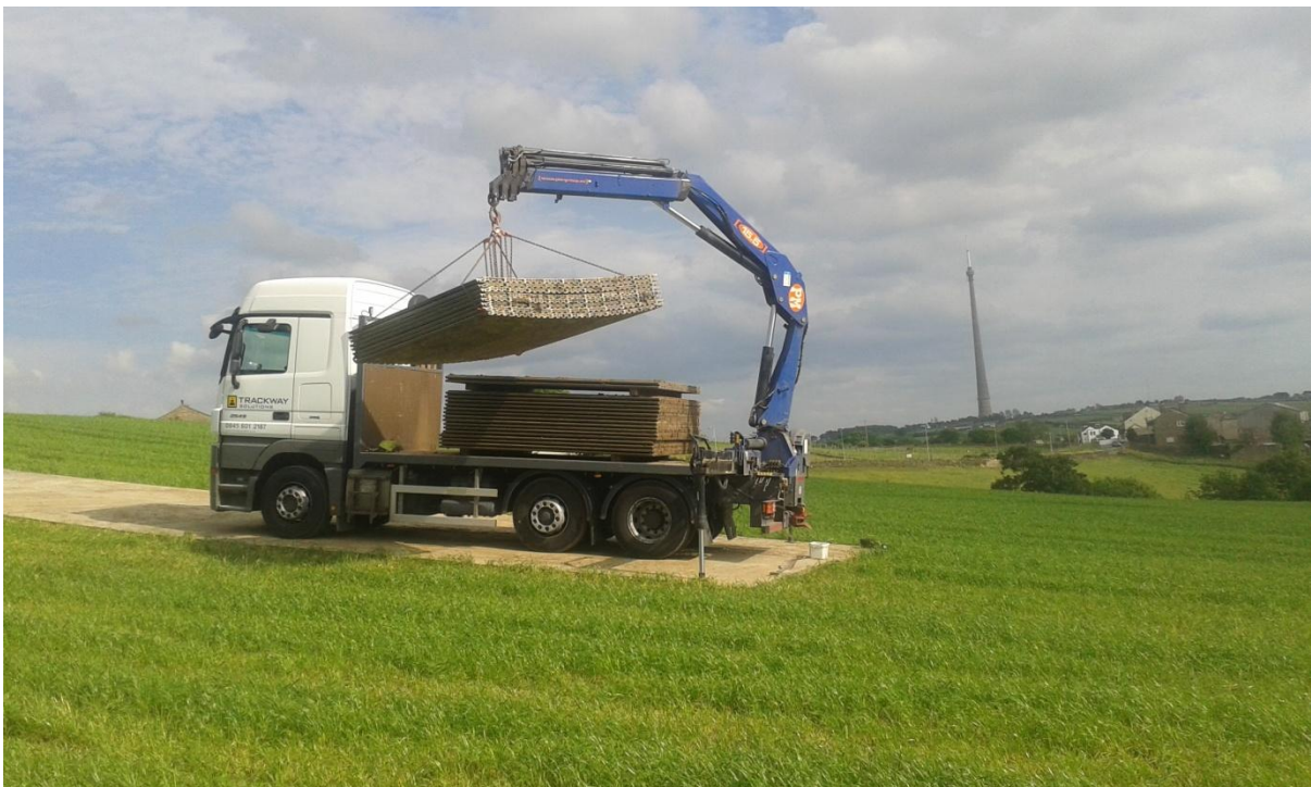
Photo 2: HGV unloading aluminium trackway
