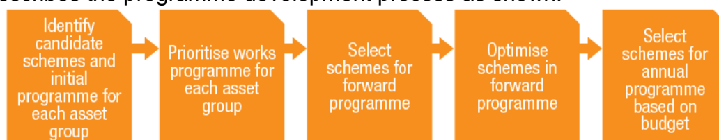
Figure 6 – Developing a Programme of Works
