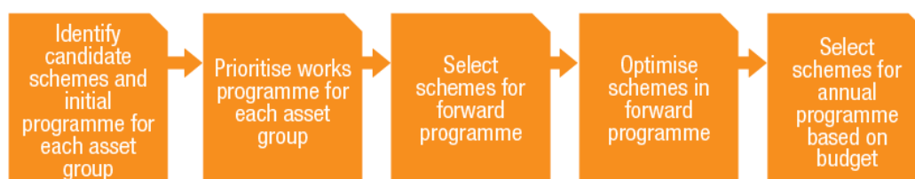
Figure 6 – Developing a Programme of Works
