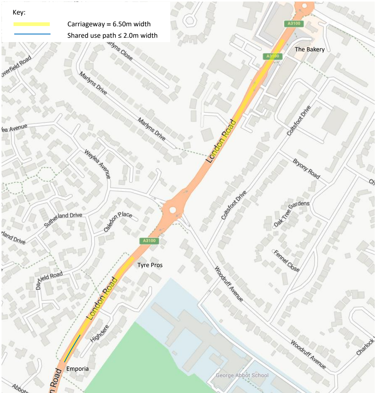
© sketched based on Bing Maps Figure 2 Extent of narrow shared use path
